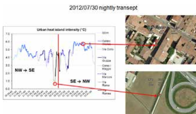
Figure 2 – UHI intensity during one nightly mobile survey. The vertical broken line indicates the U-turn during the survey
